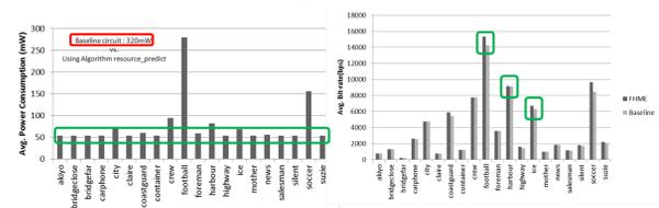
Figure 6: Motion Estimation, adapting power vs. quality using resource predict algorithm. Here, lower bit-rate implies better performance.
