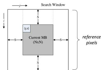
Figure 5: Fault-Handling Motion Estimation (FHME). Computation of a motion vector spatially along *j*-axis in a reference frame’s search window *S* is shown. Proposed algo can adapt *S* based on type of motion.
