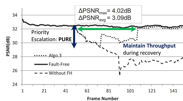
Figure 4: Fault injection and recovery in DCT module for H.263 video encoder block using different algorithms 1) FaDRes, 2) PURE. Fault-Handling Mechanism is triggered when there is a difference of 3% in PSNR (health-metric). Faults are injected in PE<sub>1</sub> (DC-coefficient) and PE<sub>4</sub>
