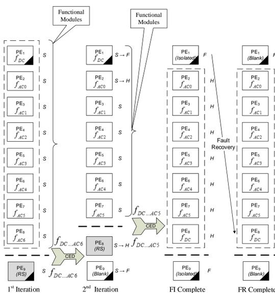
Figure 3: Fault Isolation (FI) and Recovery (FR) for 1D 8-point DCT. Here, PE<sub>1</sub> (active) and PE<sub>9</sub> (RS) are the faulty PEs which need to be identified and removed from the datapath. Initially, all resources (PEs) are deemed *suspect (S)*. FaDRes starts by identifying a *healthy RS* (2<sup>nd</sup> iteration) and then proceeds to mark resources (PEs) as *healthy (H)* or *faulty (F)*.
