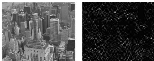
Figure 1: Health-Metric-based Fault-Handling Strategy, motivating example showing image reconstruction with (a) fully functional DCT module, PSNR=35.27dB (b) faulty PE in DCT module which computes DC-coefficient (more significant to output quality than PEs computing AC coefficients), PSNR=7.07dB.
