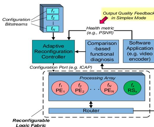
Figure 2: FPGA-based video encoder platform. ‘PSNR’ is used as a health-metric in closed loop to regulate energy/resilience/quality.
